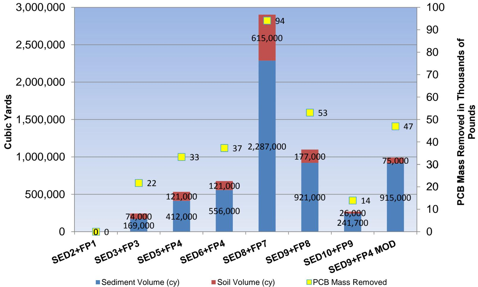
**Figure 13 - Sediment and Soil Removal Volumes and PCB Mass Removed for Combination Alternatives**
