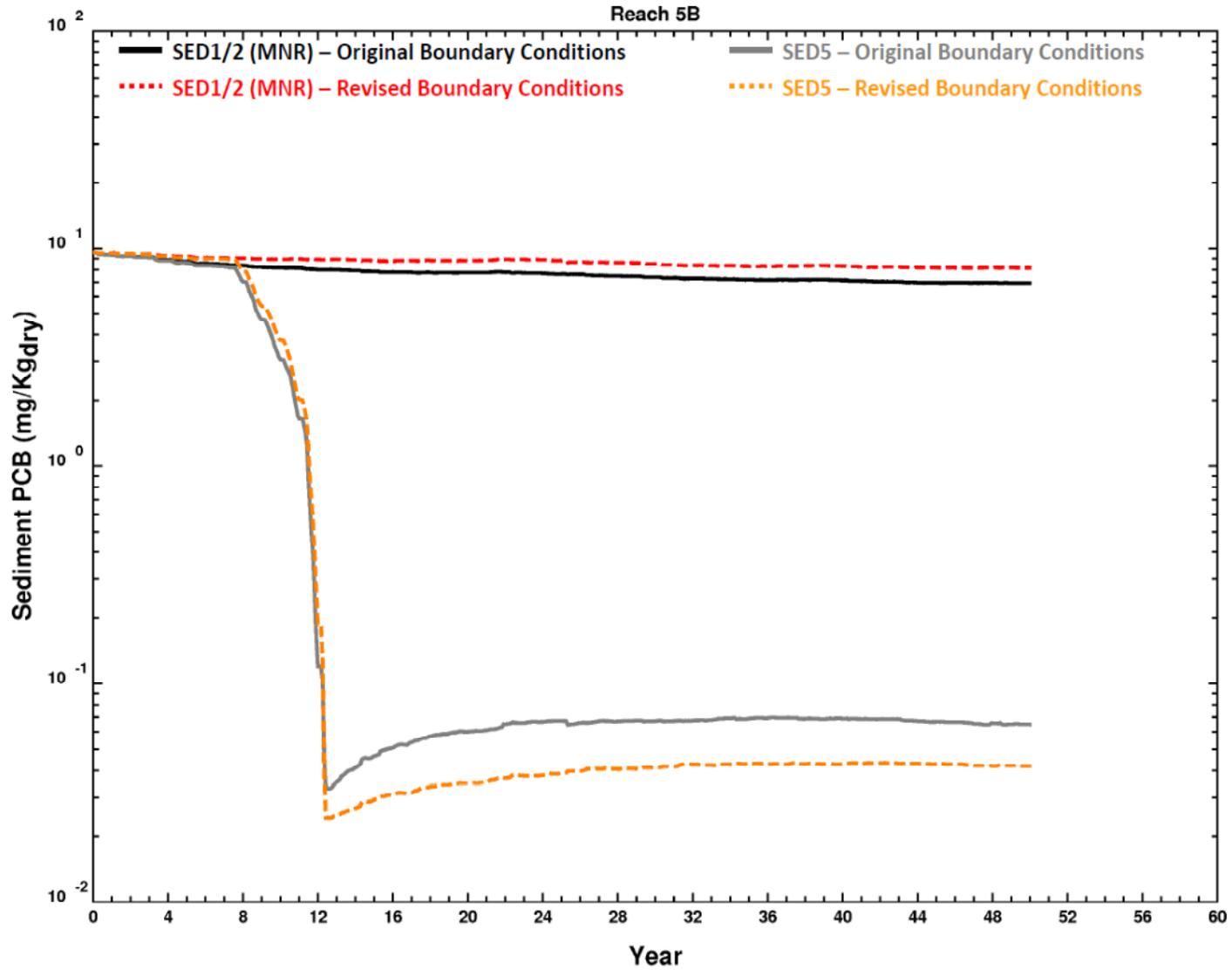
Figure 6. Reach 5B average sediment PCB concentrations from original and revised simulations
