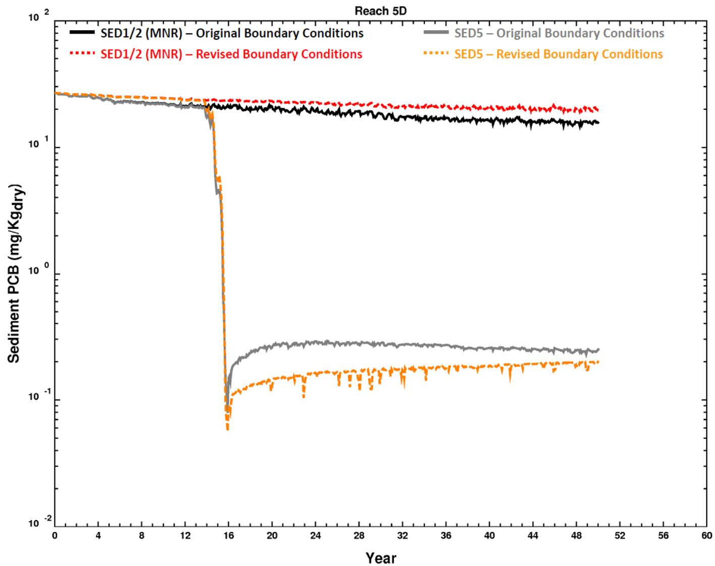
Figure 8. Reach 5D average sediment PCB concentrations from original and revised simulations
