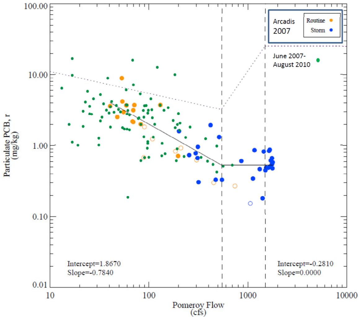
Figure 3. Additional post-remediation data (●) added to East Branch boundary particulate PCBs versus River Flow (--- Calibration/Validation, Arcadis, et.al. 2007 estimate of post-East Branch Remediation period) (Figure 4-1 of Arcadis, et.al., 2007 Supplement to Model Input Addendum) (● Routine Monitoring, ● 2007 Storm Event - GE 2007 Supplemental Monitoring Program; filled symbol = detected, open=non-detect).
