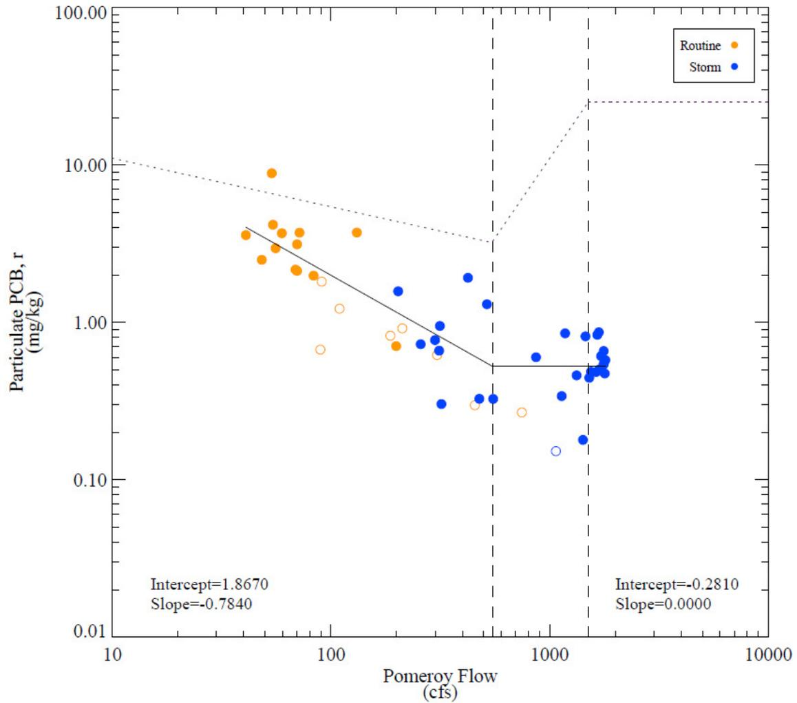
Figure 2. East Branch boundary particulate PCBs versus River Flow (--- Calibration/Validation, — Arcadis, et.al. 2007 estimate of post-East Branch Remediation period) (Figure 4-1 of Arcadis, et.al., 2007 Supplement to Model Input Addendum) (● Routine Monitoring, ● GE 2007 Supplemental Storm Event Monitoring; filled symbol = detected, open=non-detect).
