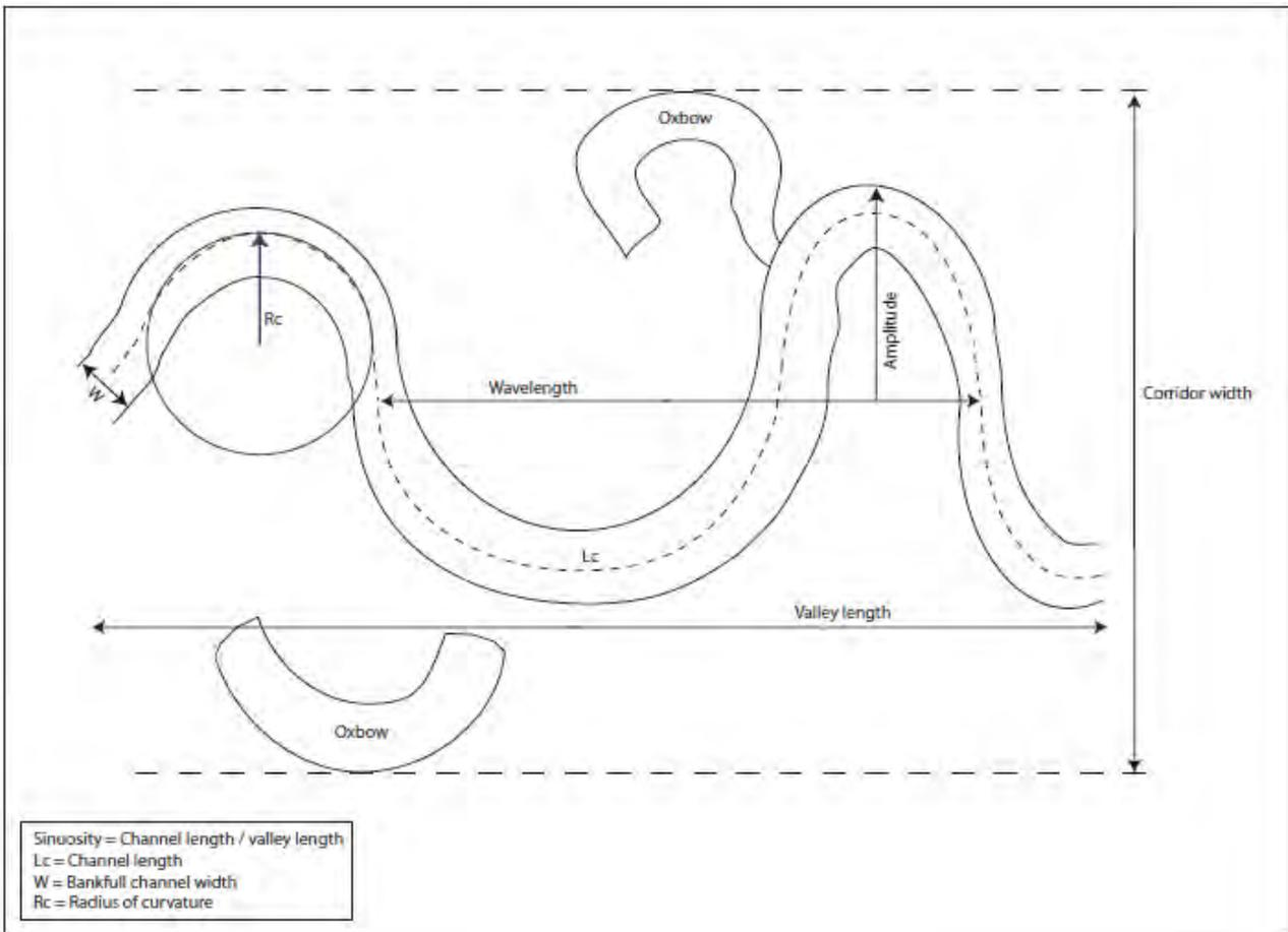
**Figure 1 Definition of Meandering Planform Characteristics**
