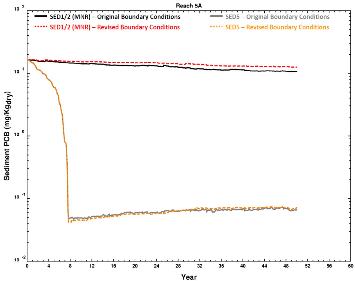
Figure 5. Reach 5A average sediment PCB concentrations from original and revised simulations
