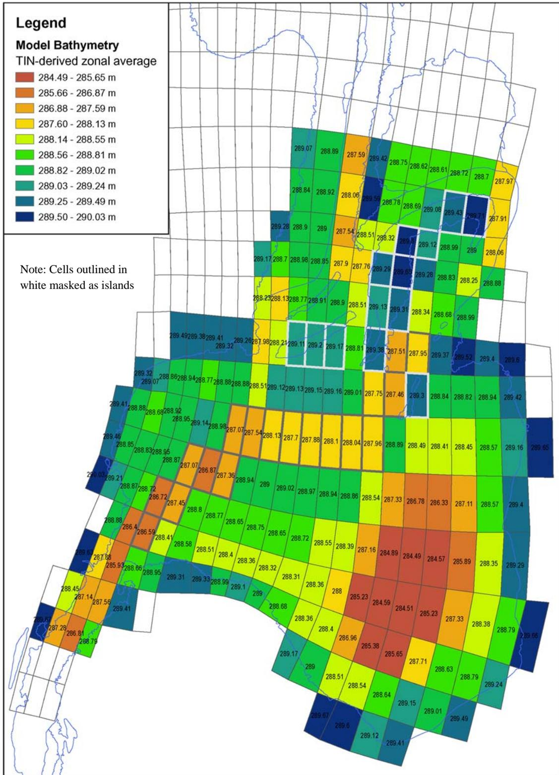
**Figure B.2-9 Model Grid in Woods Pond with Bottom Elevation Used for Each Cell**
