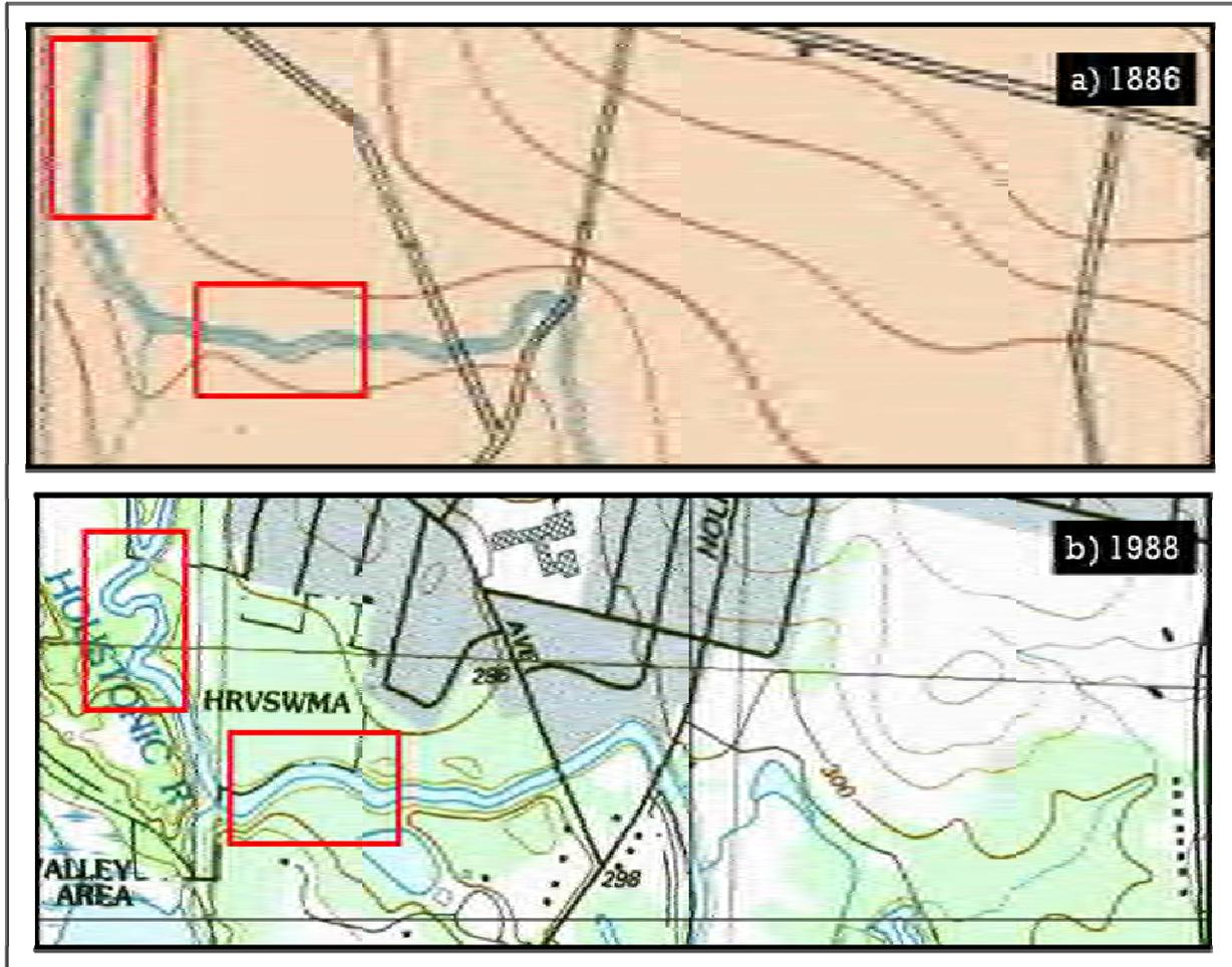
**Figure 5 Topographic Maps from a) 1886 and b) 1988 Showing the Reformation of Meanders Along an Artificially Straightened Section of the Housatonic River just Downstream of the Confluence of the East and West Branches**
