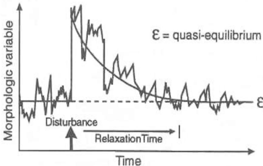
**Figure 2 Magnitude of Channel Adjustments Through Time Following a Disturbance Relative to a Quasi-Equilibrium Condition**
