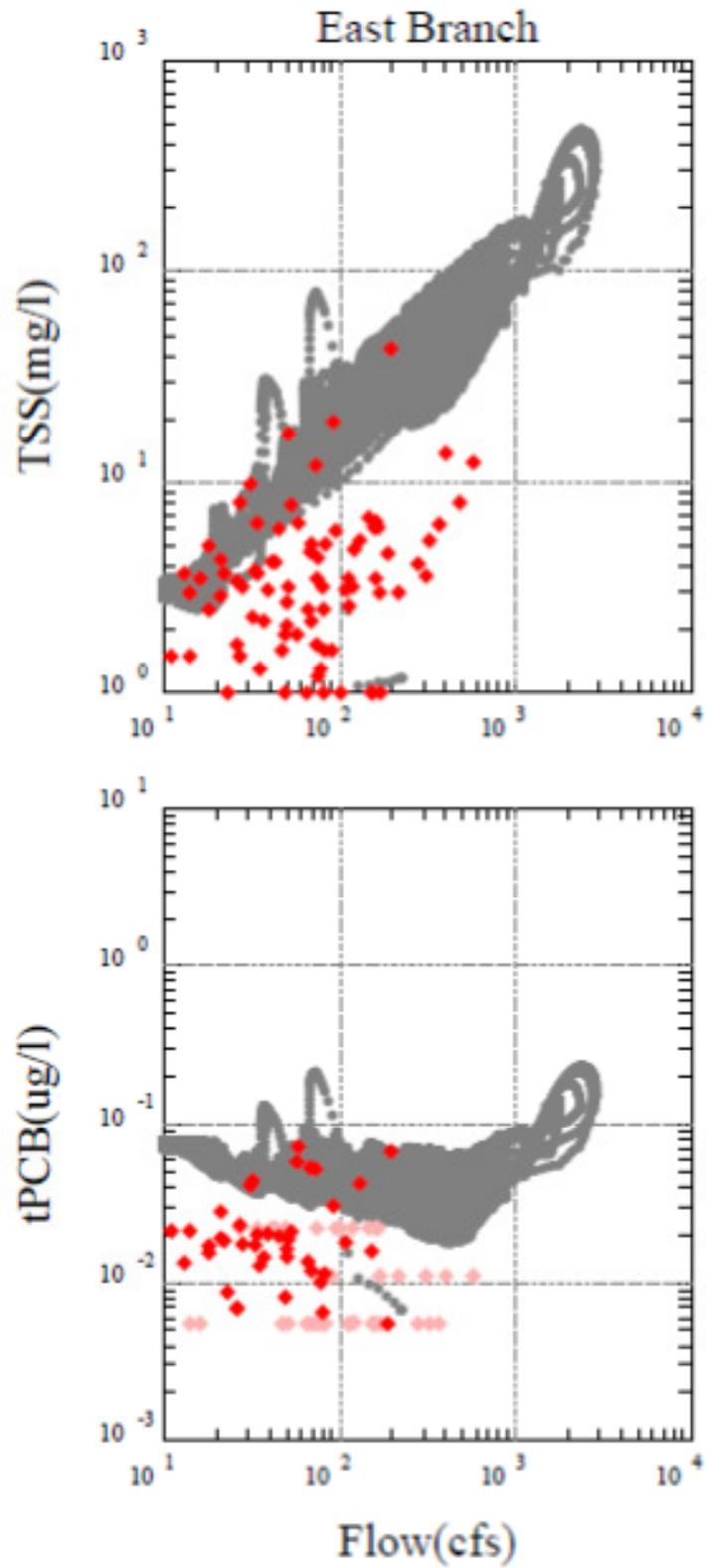
Figure 1. Comparison of original (●) TSS and PCB estimates and post-East Branch remediation period data (◆ - non-detect plotted at detection limit)
