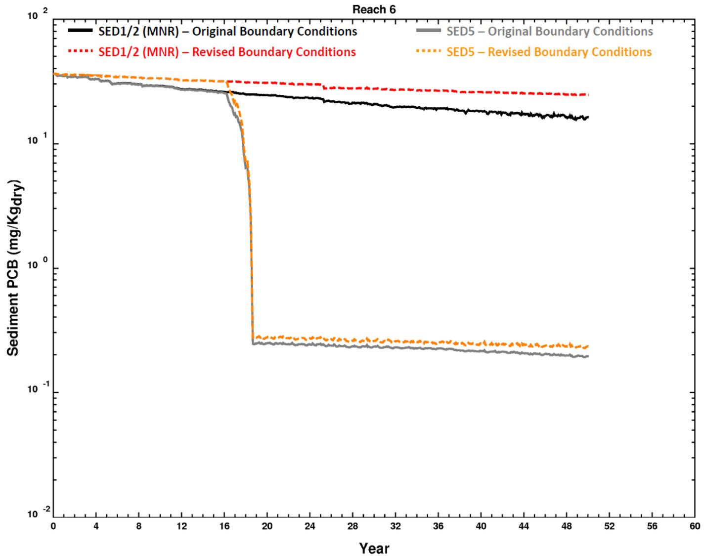
Figure 9. Reach 6 average sediment PCB concentrations from original and revised simulations
