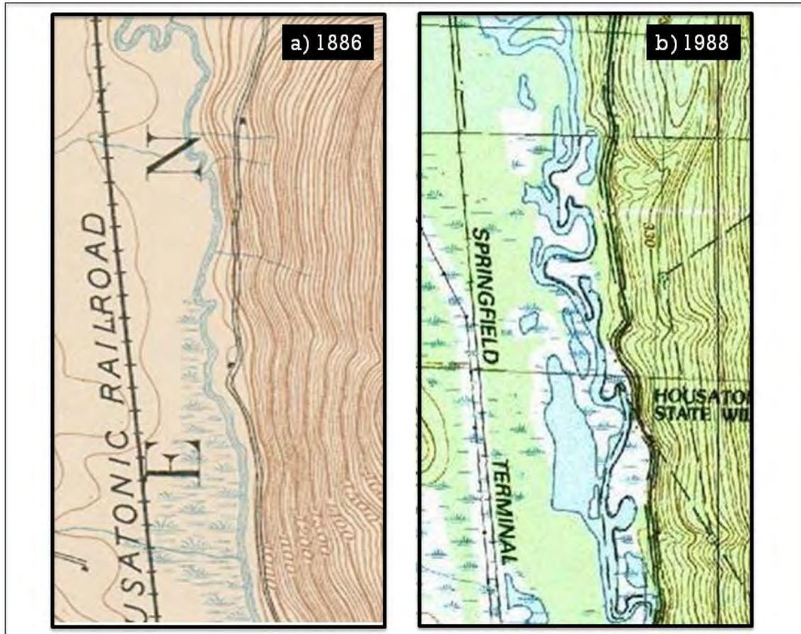
**Figure 4 Topographic Maps from a) 1886 and b) 1988 Showing Reestablishment of Meanders along an Artificially Straightened Reach of the Housatonic River just Upstream of Woods Pond**
