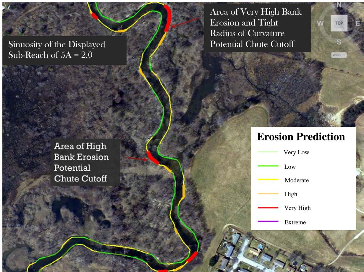
**Figure 3: Housatonic River Reach 5B - Unstable Plan Form with Tight Radii of Curvature and a High Sinuosity**
