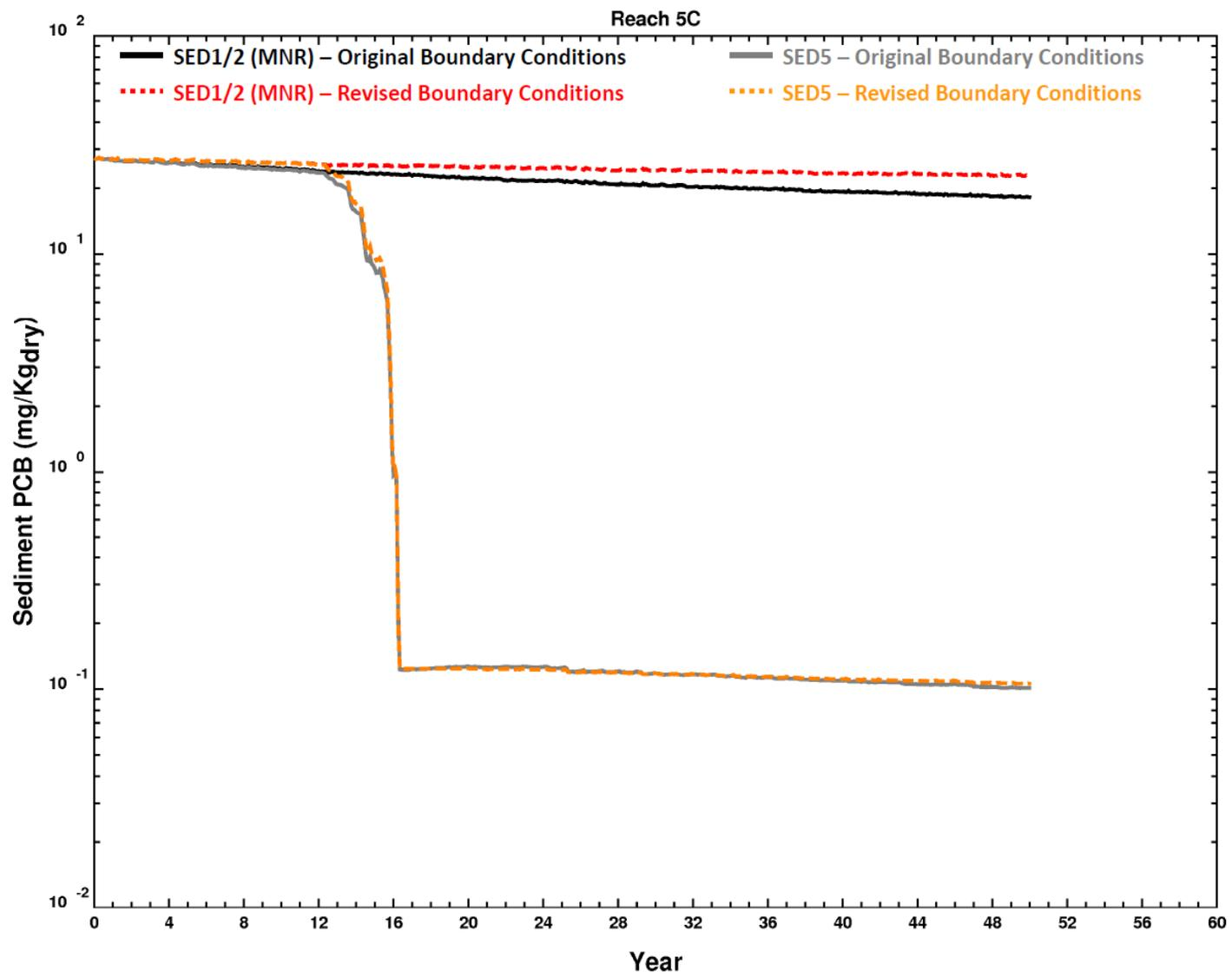
Figure 7. Reach 5C average sediment PCB concentrations from original and revised simulations
